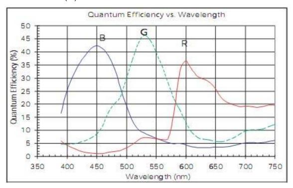
Figure1- 11 MER-500-7UC (-L) Sensor Spectral Response
