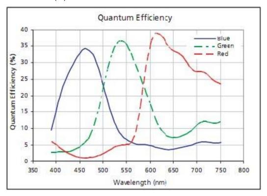
Figure1- 10 MER-310-12UC (-L) Sensor Spectral Response
