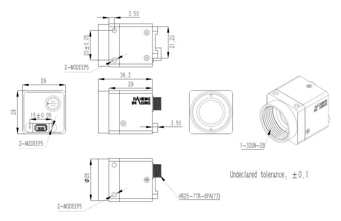
Figure2- 2 MER-U Series Mechanical Dimensions
