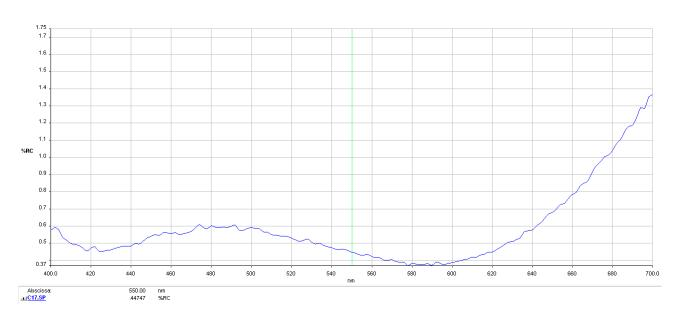
Figure2- 4 Transparent glass reflectance curve for MERCURY series mono camera
