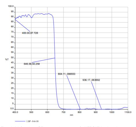
Figure 2- 3 Infrared cut-off filter transmittance curve for MERCURY series color camera
