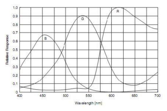
Figure1- 5 MER-125-30UC (-L) Sensor Spectral Response
