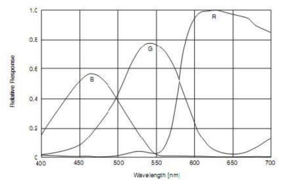
Figure1- 1 MER-030-120UC (-L) Sensor Spectral Response
