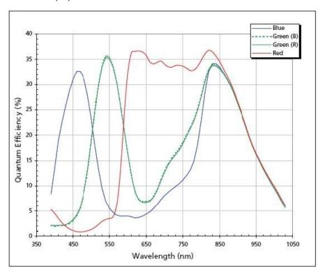
Figure1- 3 MER-040-60UC (-L) Sensor Spectral Response
