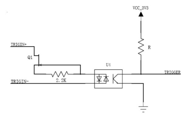
Figure 4- 2 Camera input circuit
