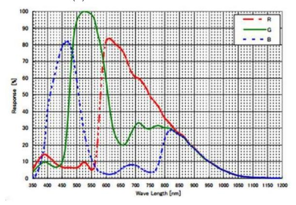
Figure1- 8 MER-132-30UC (-L) Sensor Spectral Response
