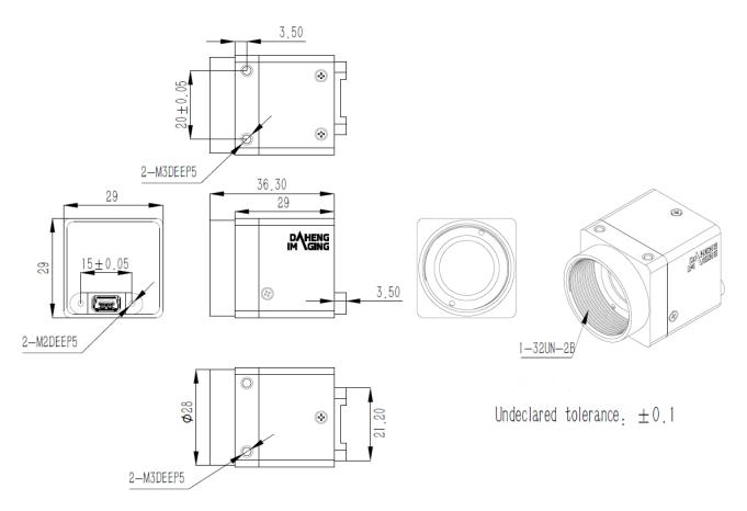
Figure2- 1 MER-U-L Series Mechanical Dimensions
