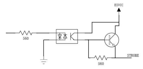
Figure 4- 3 Camera output circuit
