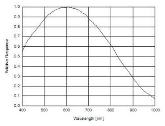
Figure1- 2 MER-030-120UM (-L) Sensor Spectral Response
