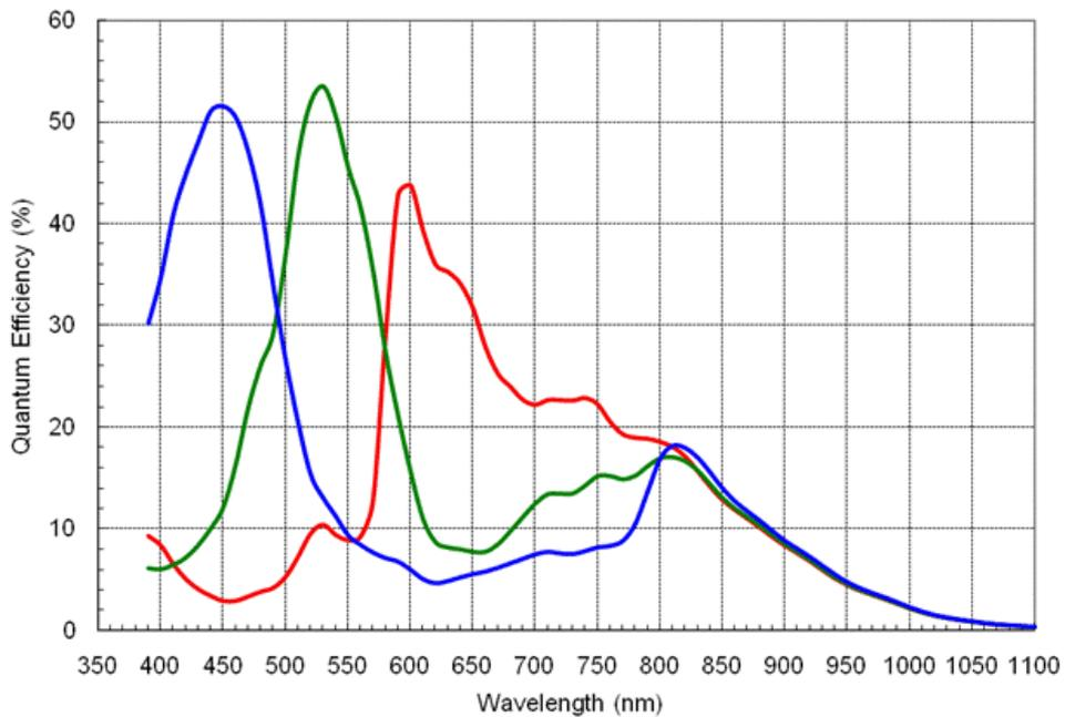
Figure 4-23 MER-500-14U3C(-L) sensor spectral response
