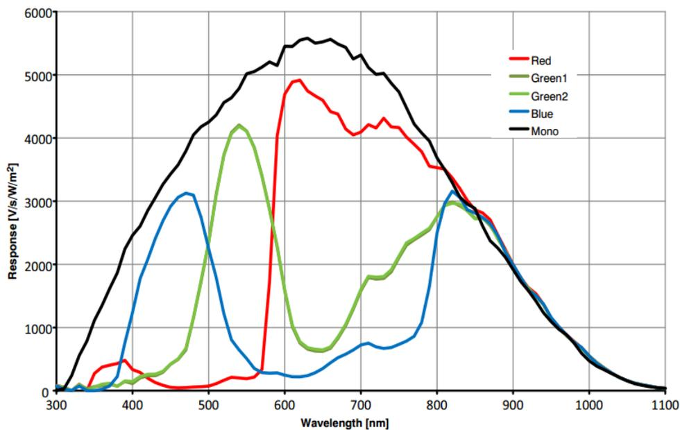
Figure 4-1 MER-031-860U3M/C(-L)/MER-050-560U3M/C(-L)/MER-131-210U3M/C(-L) sensor spectral response
