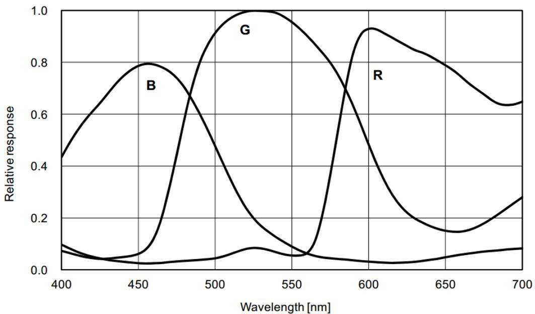
Figure 4-38 MER-2000-19U3C(-L) sensor spectral response
