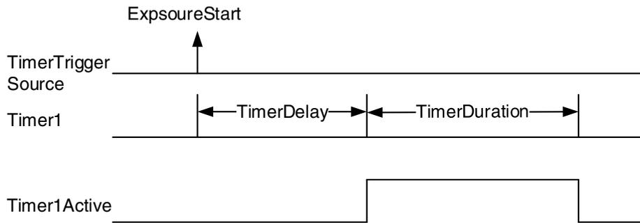
Figure 8-50 Timer1Active schematic diagram
