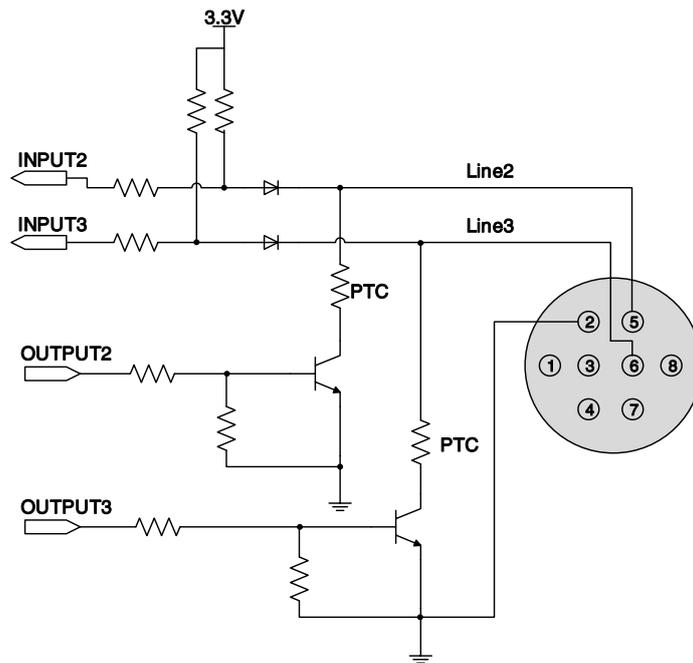
Figure 7-5 Line2/Line3 (bidirectional) circuit
