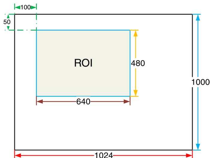
Figure 8-26 An example for the relative position between the ROI and the current image
