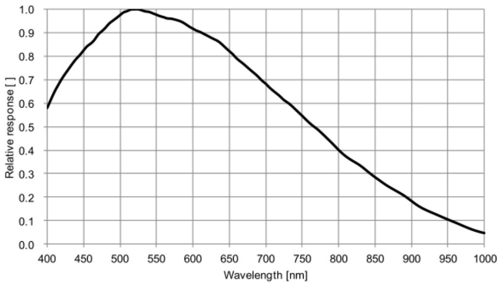
Figure 4-16 MER-231-41U3M(-L) sensor spectral response
