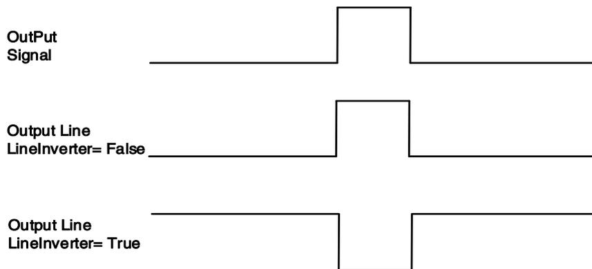
Figure 8-4 Set output line reversion
