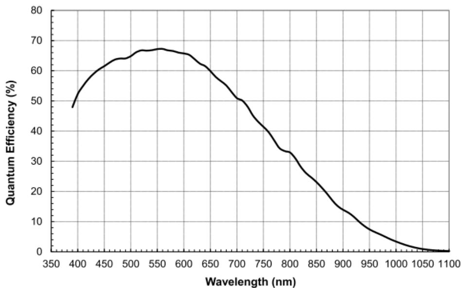
Figure 4-9 MER-133-54U3M(-L) sensor spectral response
