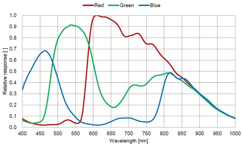
Figure 4-5 MER-041-436U3C(-L) sensor spectral response
