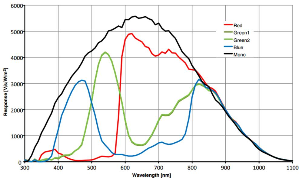
Figure 4-11 MER-134-93U3M/C(-L) sensor spectral response
