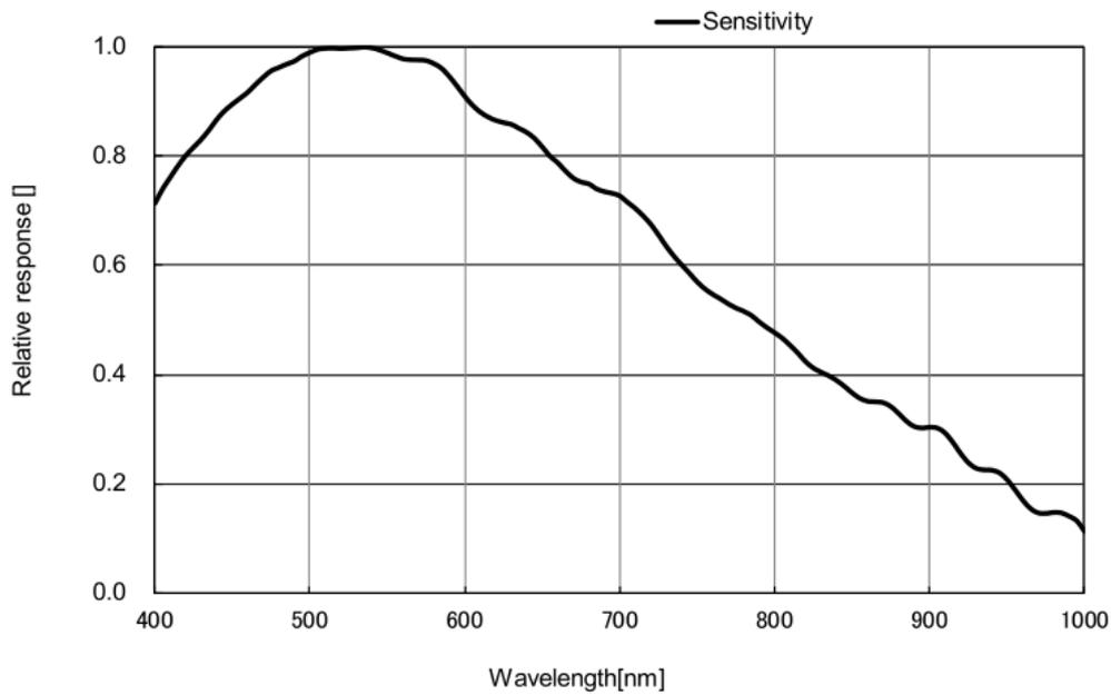
Figure 4-33 MER-1220-32U3M(-L) sensor spectral response
