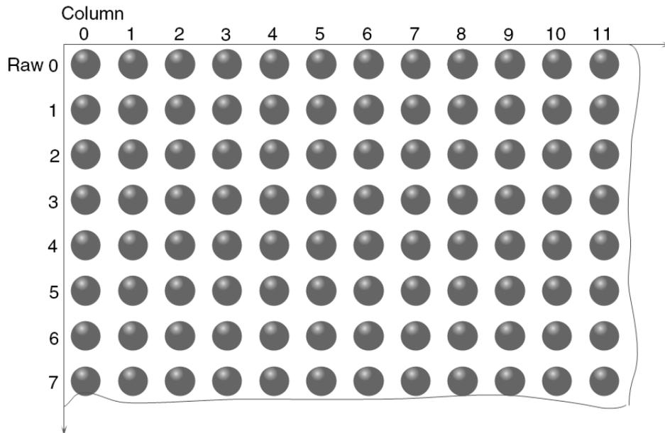
Figure 8-23 Mono8 pixel format
