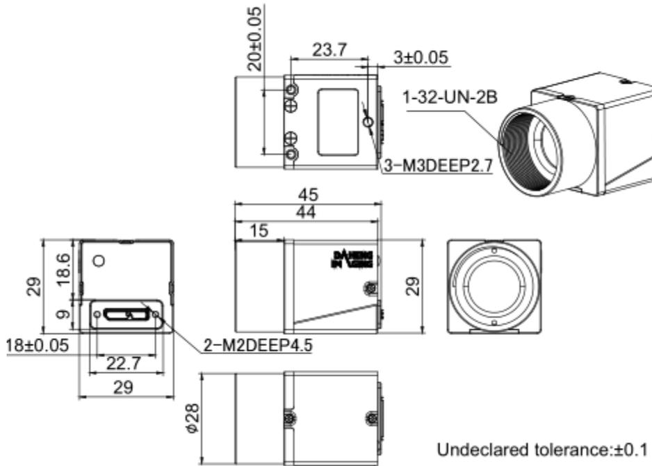
Figure 5-2 MER-U3-L mechanical dimensions
