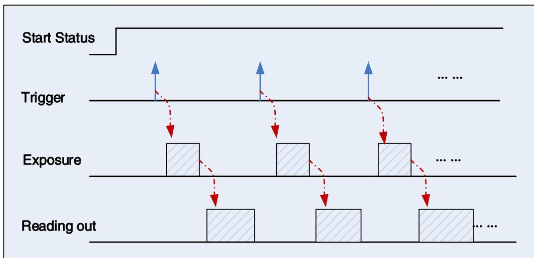
Figure 8-6 Trigger acquisition process
