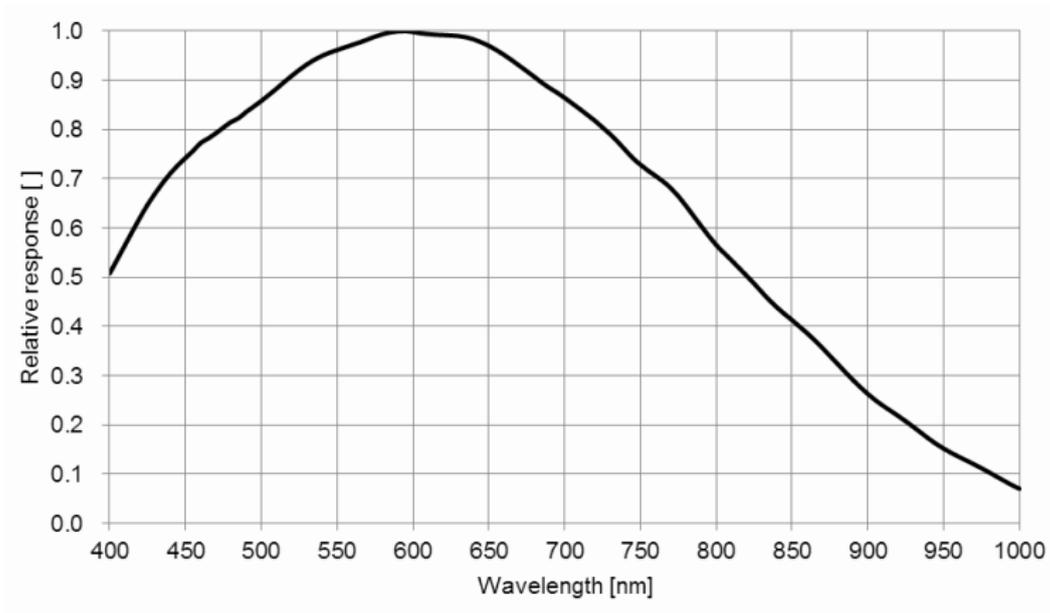
Figure 4-24 MER-502-79U3M(-L) sensor spectral response
