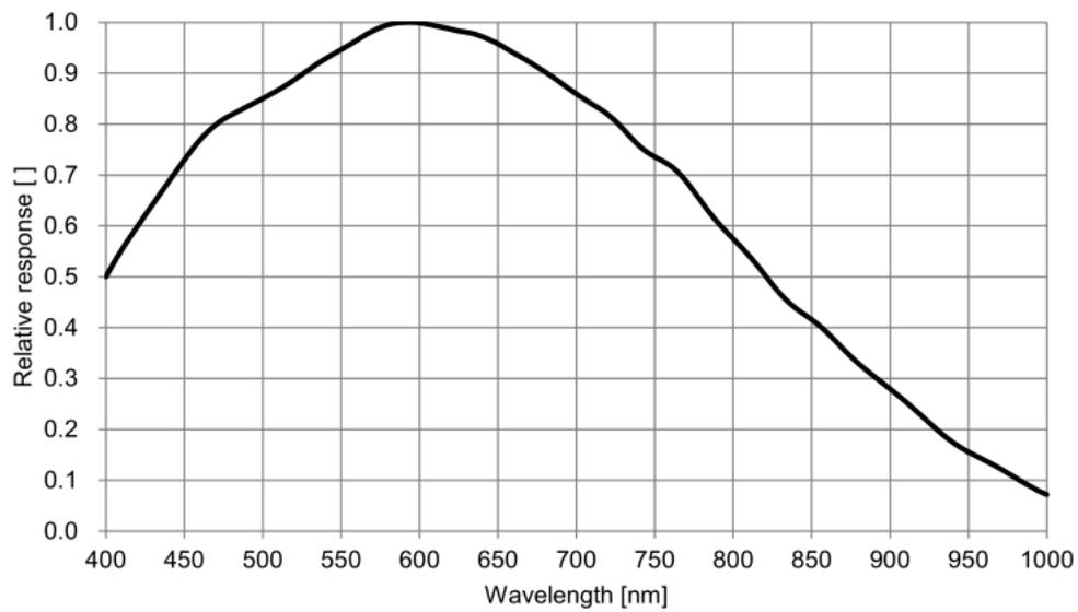
Figure 4-4 MER-041-436U3M(-L) sensor spectral response
