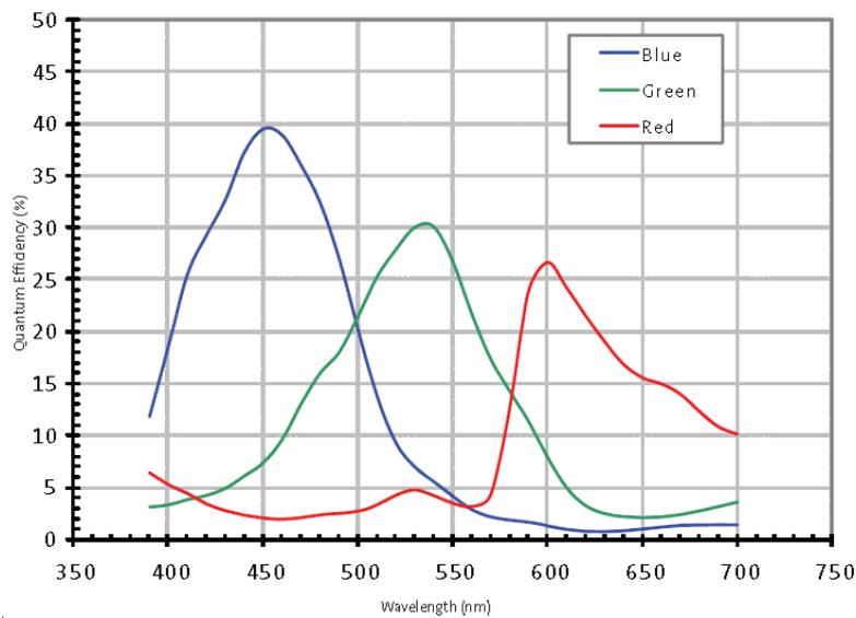
Figure 4-32 MER-1070-14U3C(-L) sensor spectral response
