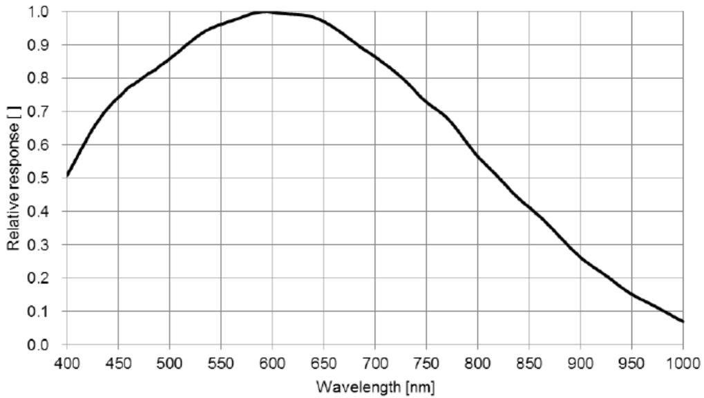
Figure 4-18 MER-301-125U3M(-L) sensor spectral response
