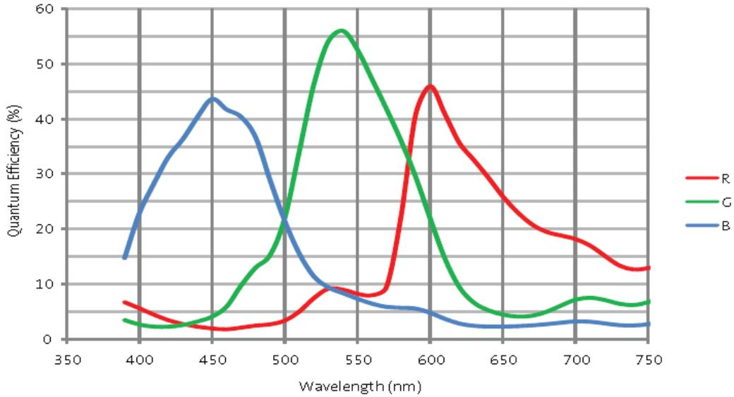
Figure 4-35 MER-1520-13U3C(-L) sensor spectral response
