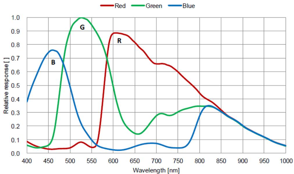
Figure 4-15 MER-230-168U3C(-L) sensor spectral response
