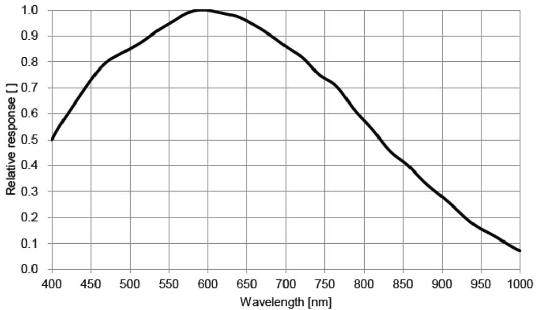
Figure 4-12 MER-160-227U3M(-L) sensor spectral response
