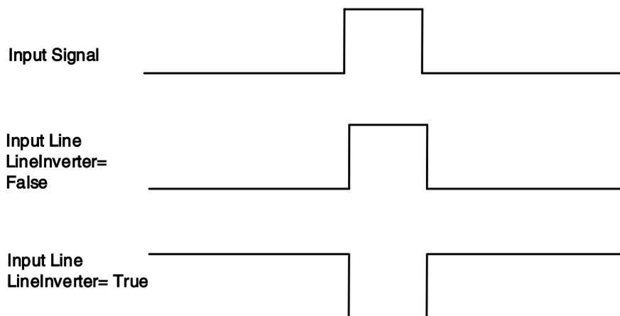
Figure 8-3 Setting input line to reverse
