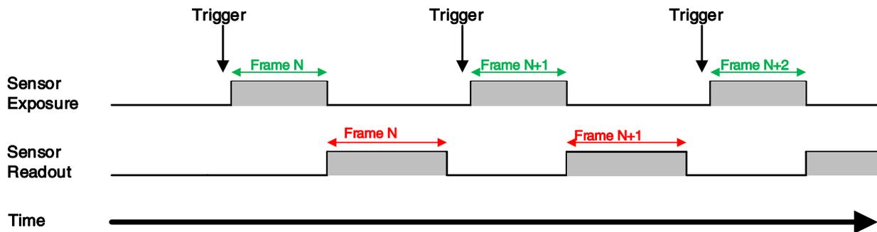
Figure 8-17 The trigger acquisition exposure sequence diagram in non-overlapping exposure mode
