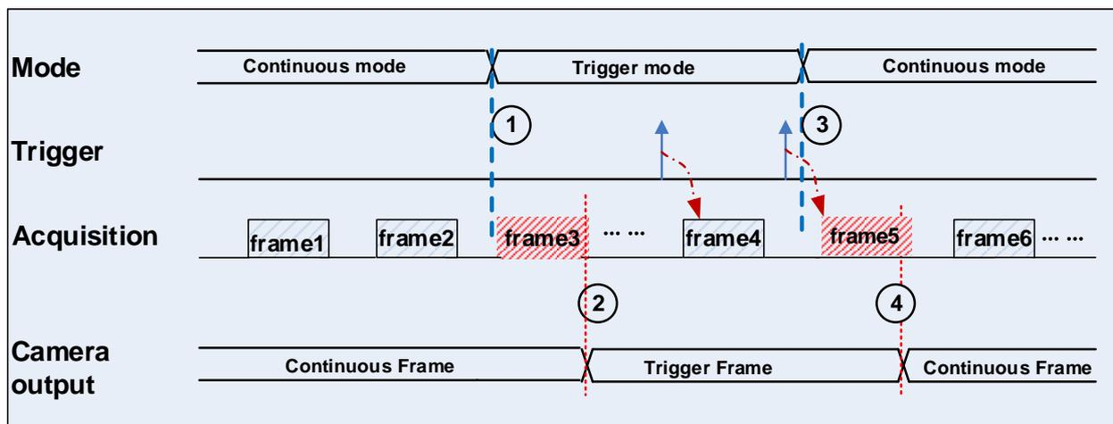
Figure 8-13 Switch acquisition mode in waiting time
