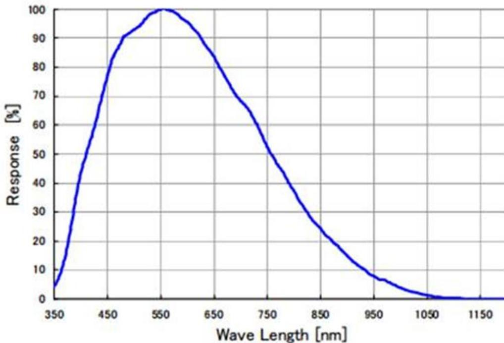
Figure 4-7 MER-132-43U3M(-L) sensor spectral response
