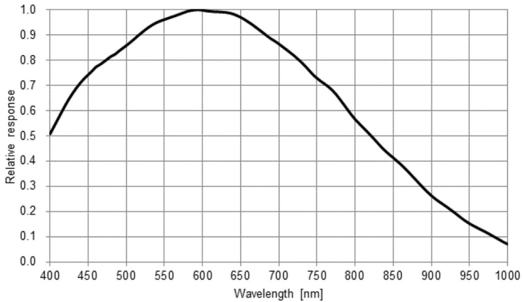
Figure 4-20 MER-302-56U3M(-L) sensor spectral response
