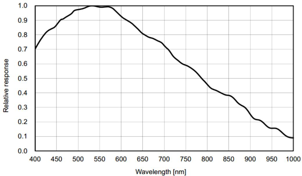
Figure 4-37 MER-2000-19U3M(-L) sensor spectral response
