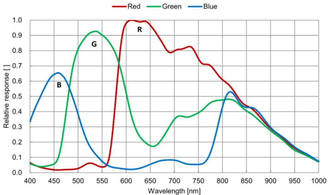
Figure 4-25 MER-502-79U3C(-L) sensor spectral response
