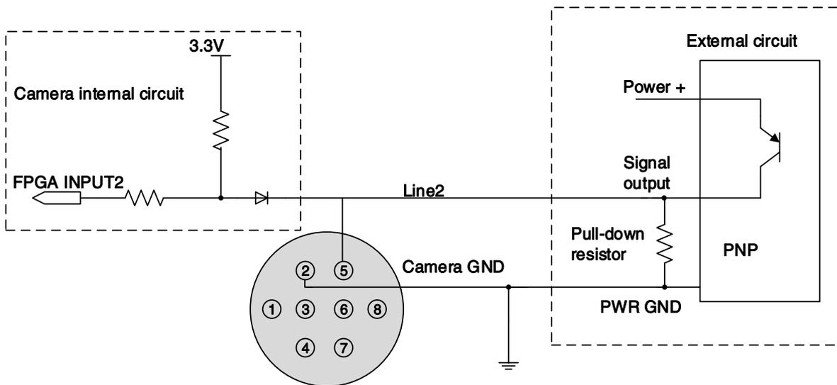
Figure 7-8 PNP photoelectric sensor connected to Line2 input circuit
