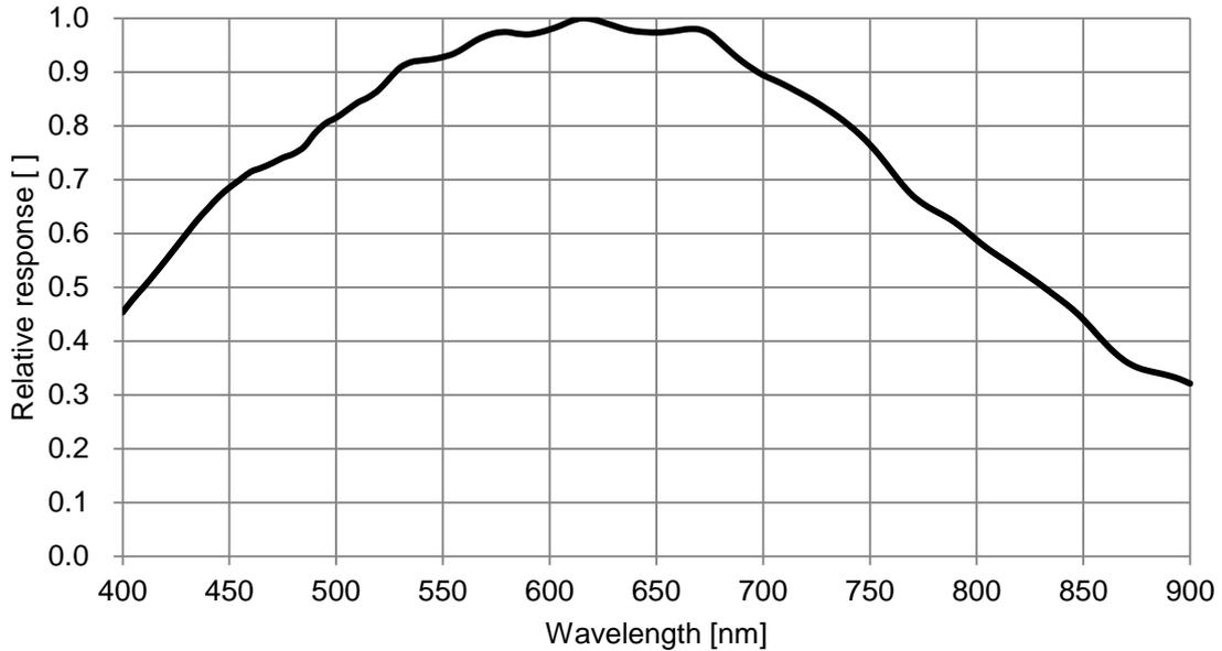
Figure 4-26 MER-502-79U3M(-L) POL sensor spectral response
