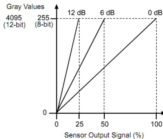
Figure 8-22 The camera's response curve
