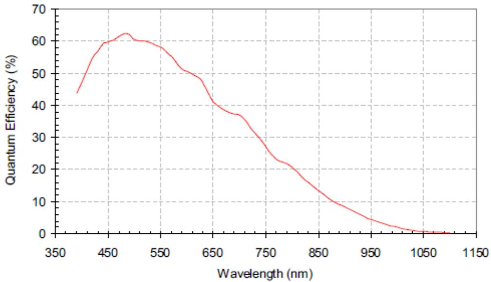
Figure 4-22 MER-500-14U3M(-L) sensor spectral response
