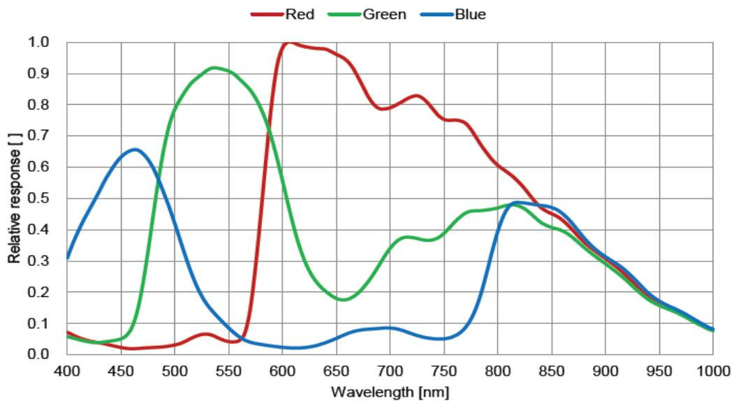
Figure 4-13 MER-160-227U3C(-L) sensor spectral response
