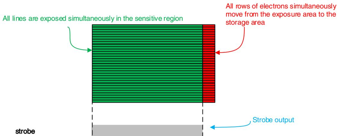
Figure 8-20 Relationship between strobe width and exposure time in global shutter exposure mode
