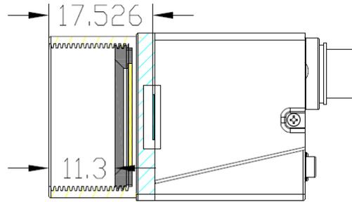
Figure 5-3 Optical interface of C-mount
