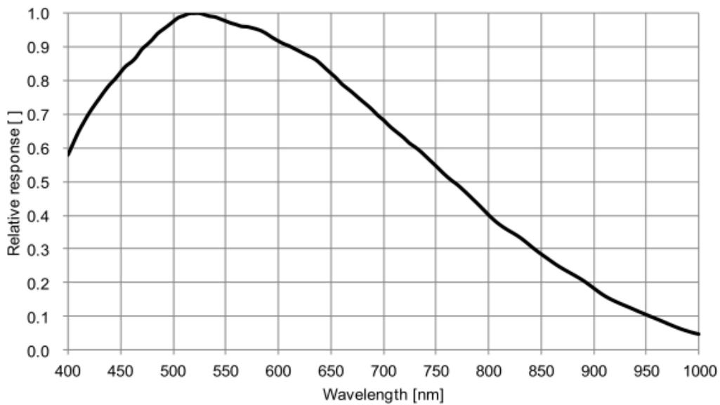
Figure 4-14 MER-230-168U3M(-L) sensor spectral response
