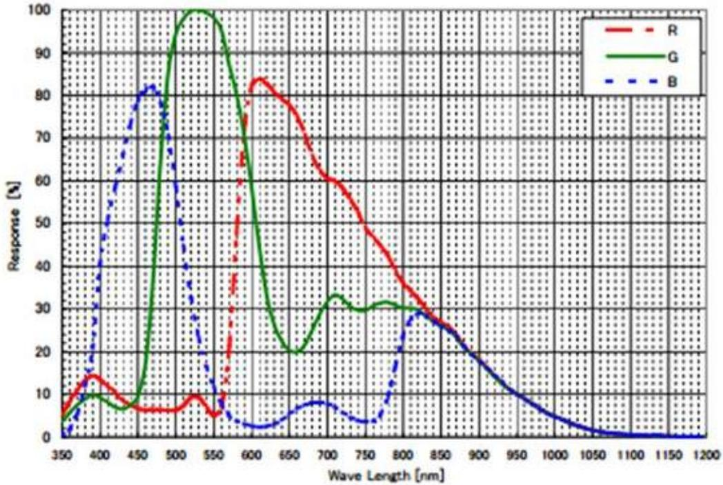
Figure 4-8 MER-132-43U3C(-L) sensor spectral response
