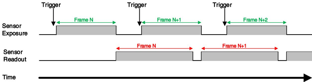
Figure 8-19 The trigger acquisition exposure sequence diagram in overlapping exposure mode
