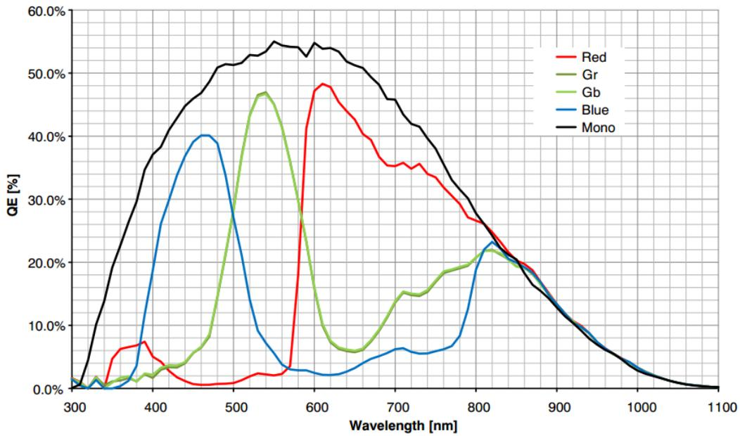
Figure 4-6 MER-051-120U3M/C(-L) sensor spectral response
