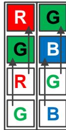
Figure 8-33 Vertical color Binning by 2
