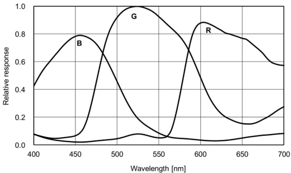
Figure 4-34 MER-1220-32U3C(-L) sensor spectral response
