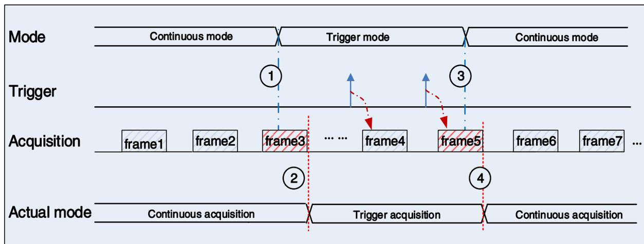
Figure 8-12 Switch acquisition mode during reading out
