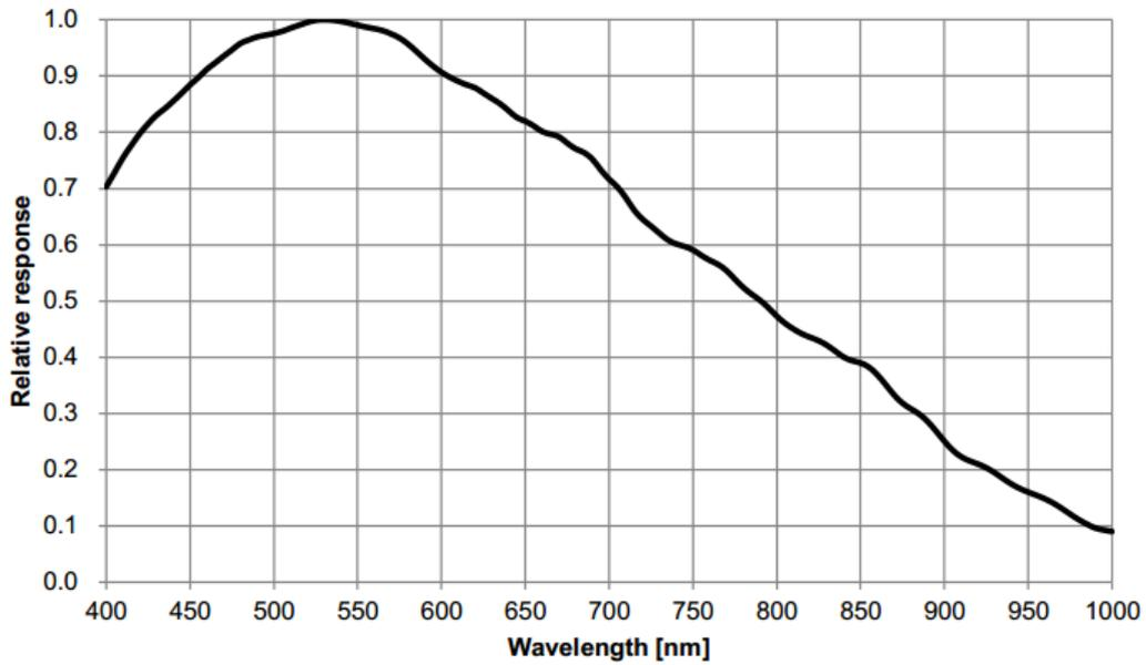
Figure 4-29 MER-630-60U3M(-L) sensor spectral response
