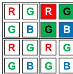
Figure 8-34 Horizontal and vertical color Binning by 2x2
