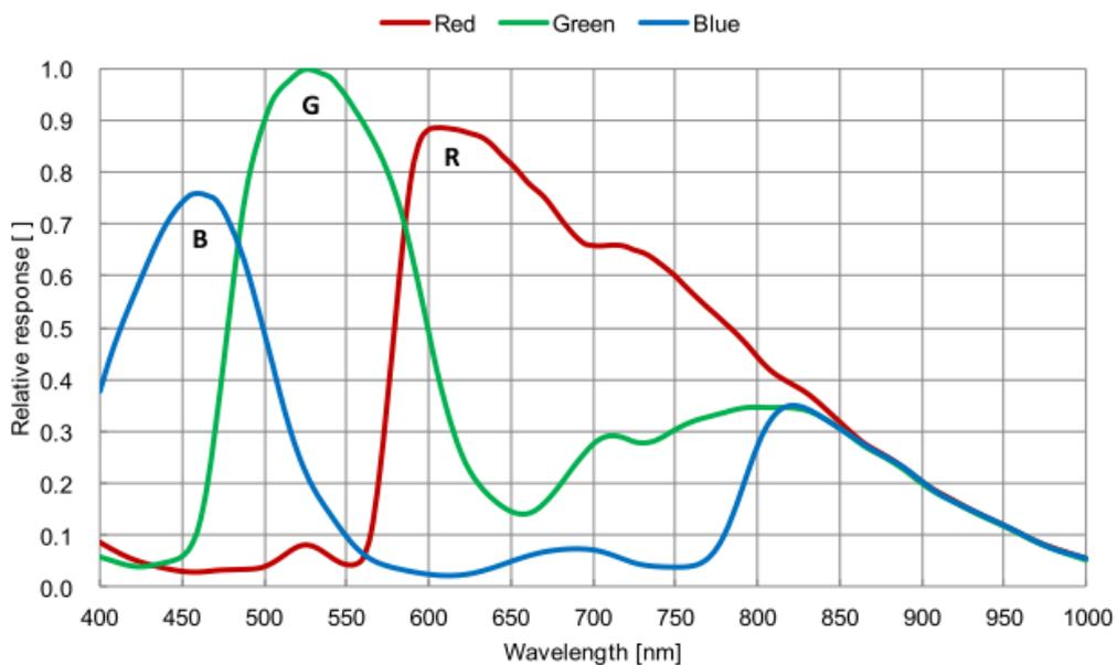
Figure 4-17 MER-231-41U3C(-L) sensor spectral response
