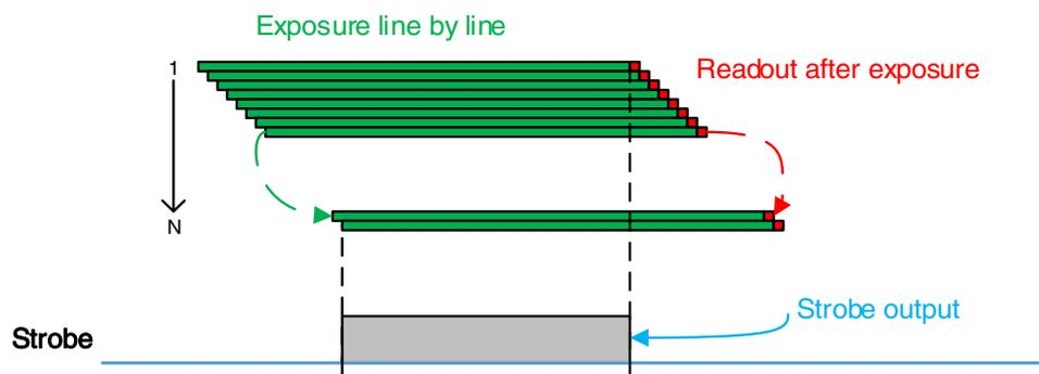
Figure 8-21 Relationship between strobe width and exposure time in rolling shutter exposure mode
