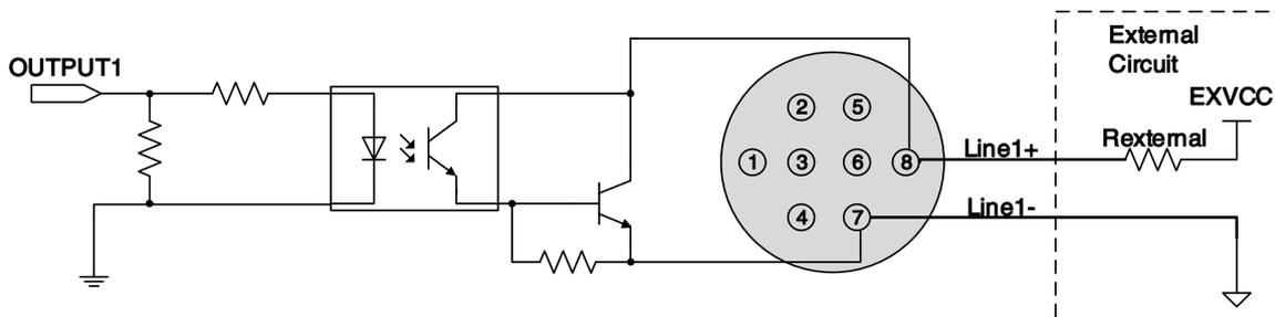
Figure 7-3 Opto-isolated output circuit
