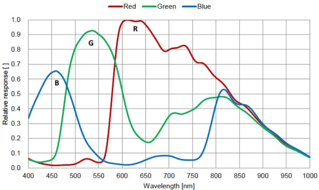
Figure 4-19 MER-301-125U3C(-L) sensor spectral response
