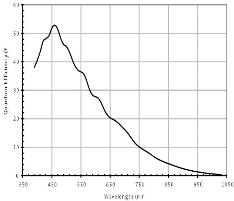
Figure 4-31 MER-1070-14U3M(-L) sensor spectral response
