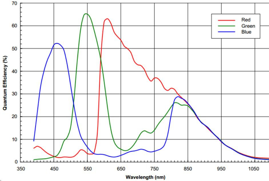
Figure 4-10 MER-133-54U3C(-L) sensor spectral response
