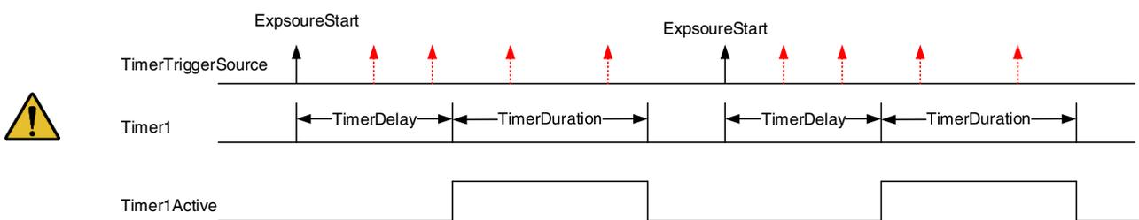
Figure 8-51 The relationship of Timer1Active and ExposureStart signal
