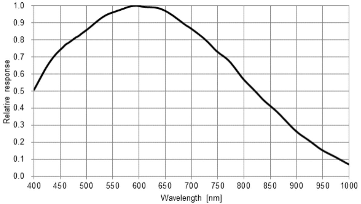
Figure 4-27 MER-503-36U3M(-L) sensor spectral response
