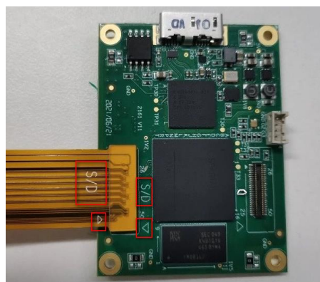
Figure 3-5 The mark of the FPC cable and the connector of the acquisition board
