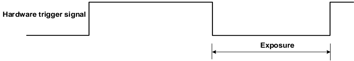
Figure 8-26 The sequence diagram in falling edge trigger of TriggerWidth exposure mode
