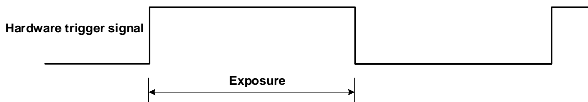
Figure 8-25 The sequence diagram in rising edge trigger of TriggerWidth exposure mode
