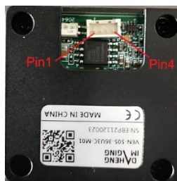
Figure 7-1 I/O interface of all-in one USB3.0 camera
