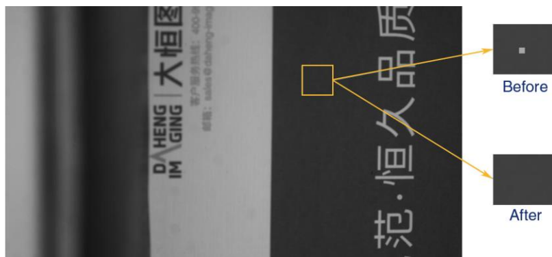
Figure 8-65 Defect pixel correction effect in actual scenario
