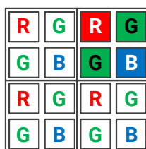
Figure 8-49 Horizontal and vertical color Binning by 2x2
